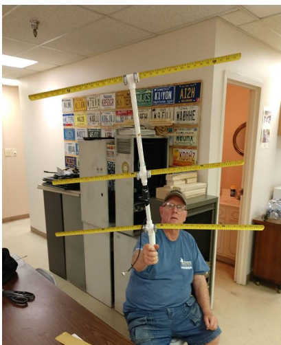
S a n d y / KM4PJU with the Tape Measure antenna he constructed at the Club
