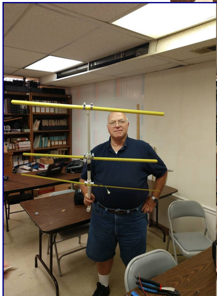
Bart/KB4FEE with the Tape Measure antenna he constructed at the Club shack.
