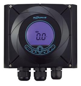
INJ-4500L is a single phase specific pump VFD which adjusts the pump speed to maintain constant pressure to max. energy saving. The drives can be applied for residential and commercial water supply, water treatment etc. As the drives are self-cooling and motor-independent structure, it can be installed directly on the motor.
