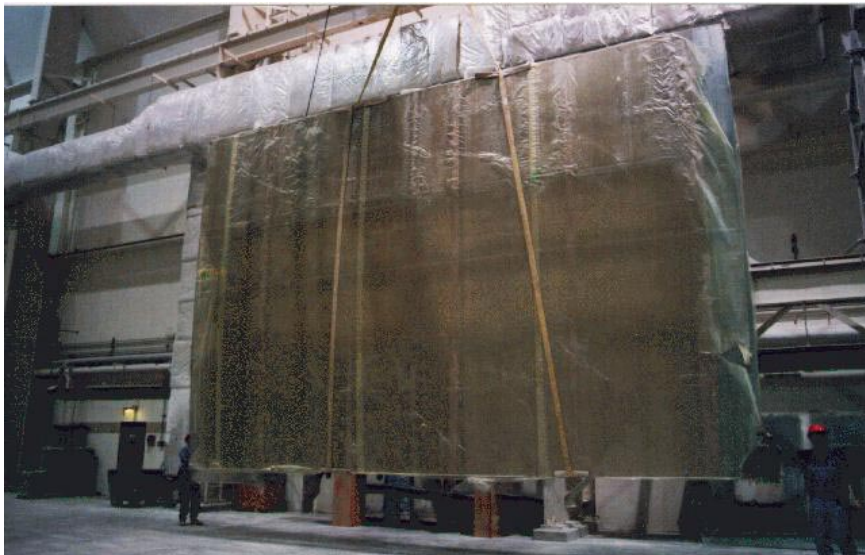
Figure 7 Main deck being moved off mold
