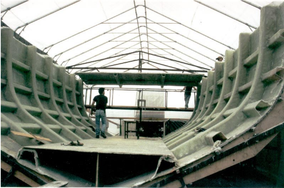
Figure 9 Installation of stiffeners and deck plates
