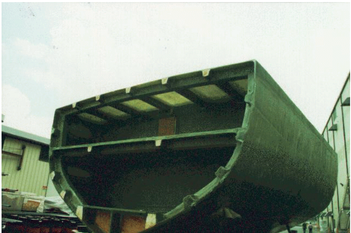
Figure 10 Completed Hull test Section
