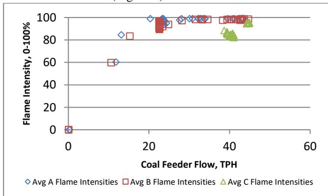
Fig. 7. Average flame intensities measured for A, B and C pulverizer burners in service from full load to 180 MWg.
