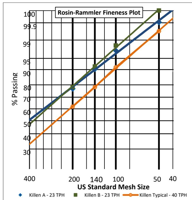
Fig. 8. Fineness Results from A and B Pulverizers
