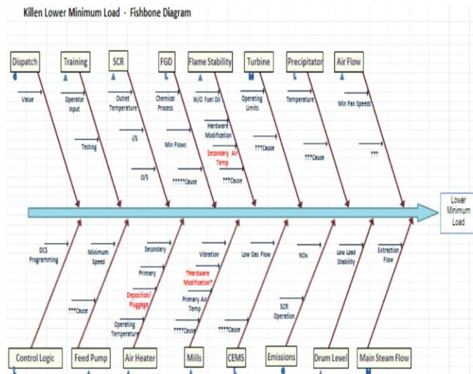
Fig. 5. Low Load Fishbone Diagram
