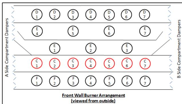
Fig. 2. Front wall burner configuration
