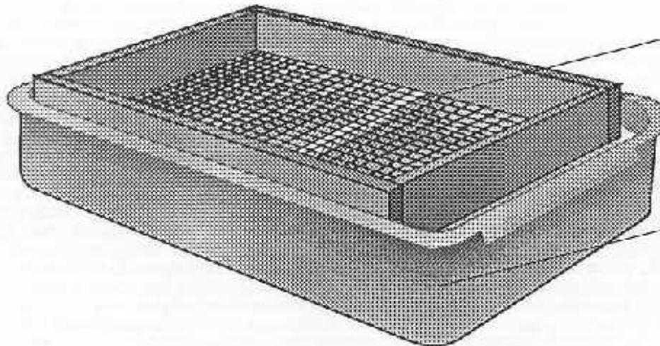
$\frac{1}{2}$ " hardware cloth screen framed by  $\frac{3}{4}$  x 2" wood to receive sample, outside dimensions of frame  $11 \frac{3}{4}$  x  $15 \frac{7}{8}$ "
