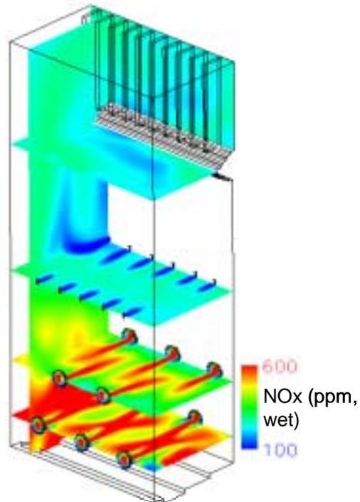
**Figure 10. Predicted NOx concentration profiles for OFA Case1.**
