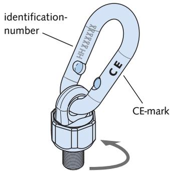
**Application:** The HD Rotary head lifting link can be used for diagonal as well as for shear loads. The rotatable head facilitates insertion into the anchor; the HD Rotary head link can be screwed into the HD Anchor while still attached to the crane hook.
