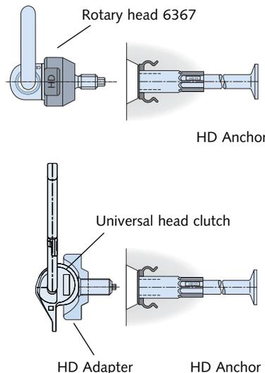
Alternatively, if a spreader beam is not available it is possible to use the rotary head lifting link 6367 or the HD Adapter no. 6366 in combination with the universal head link no. 6102.
