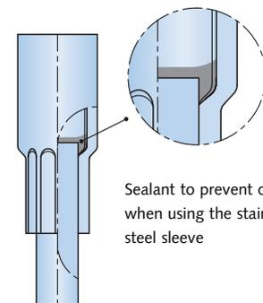
Sealant to prevent corrosion when using the stainless steel sleeve
