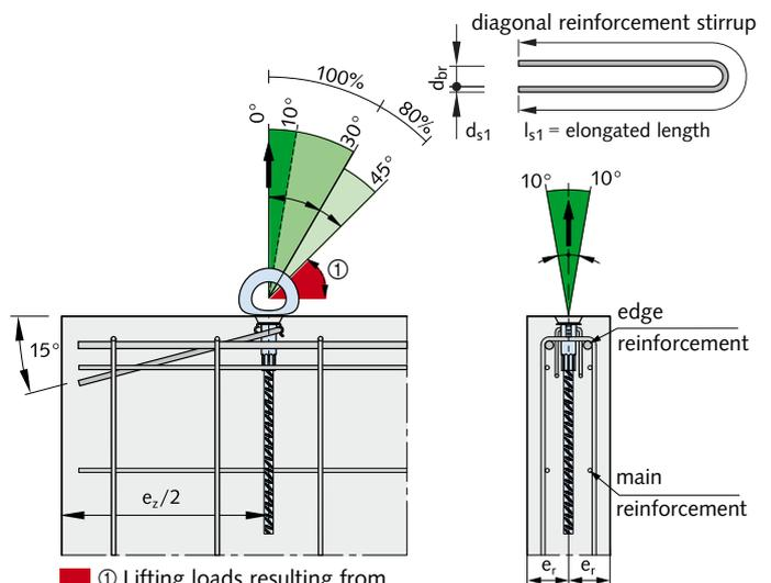
① Lifting loads resulting from cable spread within this (angle) range is not permitted.
