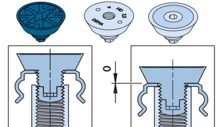
**!** Identification caps are packed separately. These must be fitted to the appropriate HD Anchor which has the same identification colour. The integrated thread protection remains in the HD Anchor permanently (Fig. 4).
