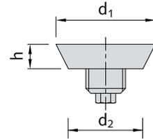
Plastic nailing plates are used to attach HD Anchors to formwork; they are available for thread sizes from Rd 12 to Rd 52.
