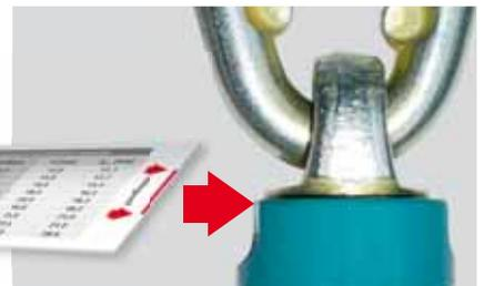
**Check wear using the check-card/0.5 mm** Discard the anchor if the card can be inserted deeper than the red line (as illustrated).
