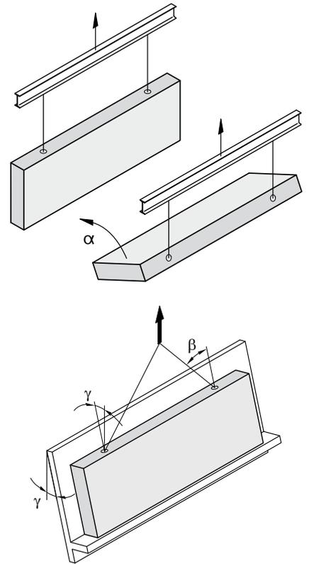
The shear reinforcement can be omitted when using a tilting table and a load angle of  $\gamma < 15^\circ$ .
