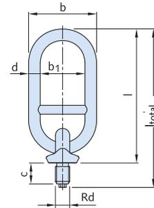
**!** The threads must be checked regularly for damage. Recutting threads is not permitted.
