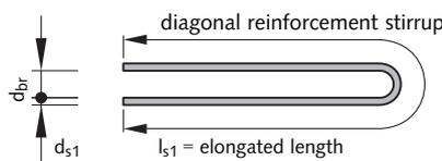
The bending roll diameter according to EC2 may be disregarded.
