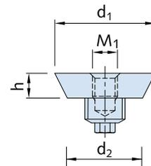
The resulting recess fits the shape of the HD Lifting link exactly. The shape of the recess allows the lifting link to distribute shear or diagonal load more effectively into the concrete.
