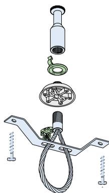
Cable loop with securing bracket (5.0 - 25.0 kN)
