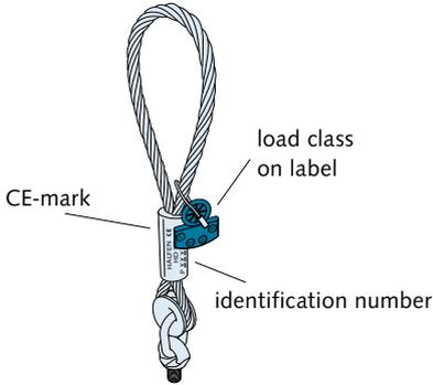
**Application:** The HD Perfect head lifting clutch is especially suited for diagonal loads and is used for lifting wall elements upright with load angles under 90°. Observe the application instructions for HD Anchors!
