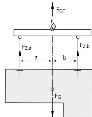
The centre of gravity of the load will always stabilise vertically under the crane hook. Load distribution in non-symmetrical installed anchors when using a spreader beam is calculated as follows:
