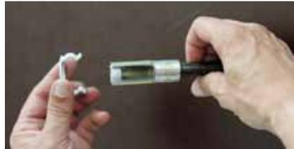
**Steel nailing plates:** The sleeve protection cap is turned inwards while screwing the assembly onto the steel nailing plate (see cut-away below).
