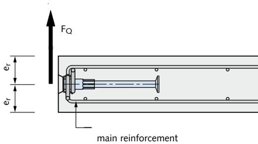
The shear reinforcement on both sides also serves as diagonal load reinforcement. Additional diagonal load reinforcement is not required.
