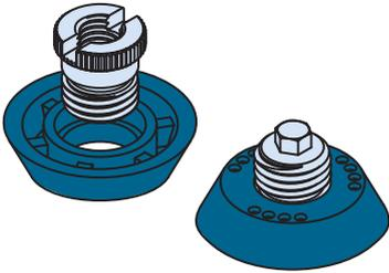
The HD Nailing plate which consists of a steel core and a replacement ring is used for fixing a HD Anchor to the formwork. Available in thread sizes Rd 12 to Rd 64.
