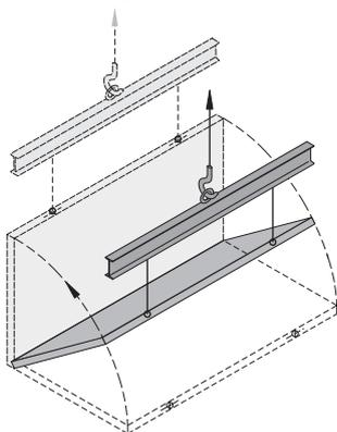
The shear reinforcement on both sides also serves as diagonal load reinforcement. Additional diagonal load reinforcement is not required. The additional shear reinforcement must be installed with full contact to the threaded socket.
