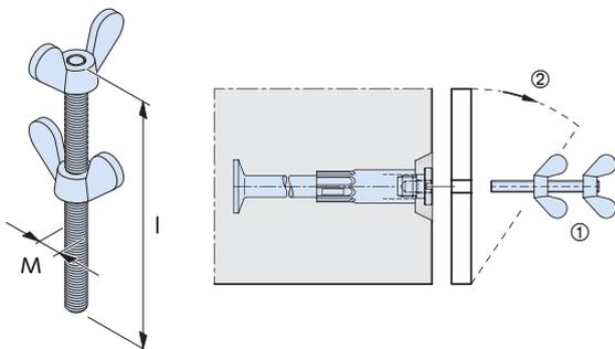
The retaining bolt is used to attach the steel nailing plate. A butterfly bolt is crimped to one end to tighten the bolt; an additional butterfly bolt is used to secure the bolt to the formwork.
