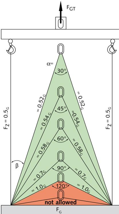
■ This spread angle is not permitted for cable spread!
