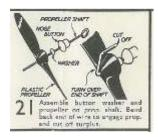
No changes to step 21. The original kit came with a six inch propeller.
