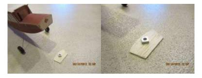
There are many ways to make a removable nose piece. I like to use a square nut cemented to the nose piece. This has several advantages:
