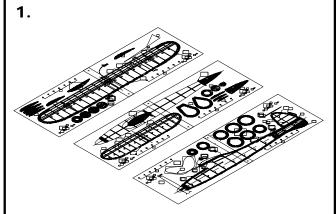
Tape the six plan pages together to form three building plan pages. Use the "+" marks for alignment of the pages.
