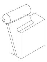
It is suggested that the prop hanger be printed in the orientation shown. Supports are not required. Also use the minimum layer height allowed for your printer.
