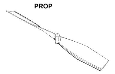
It is suggested that the prop be printed with the forward face down. Use slicer generated supports. Also use the minimum layer height allowed for your printer.
