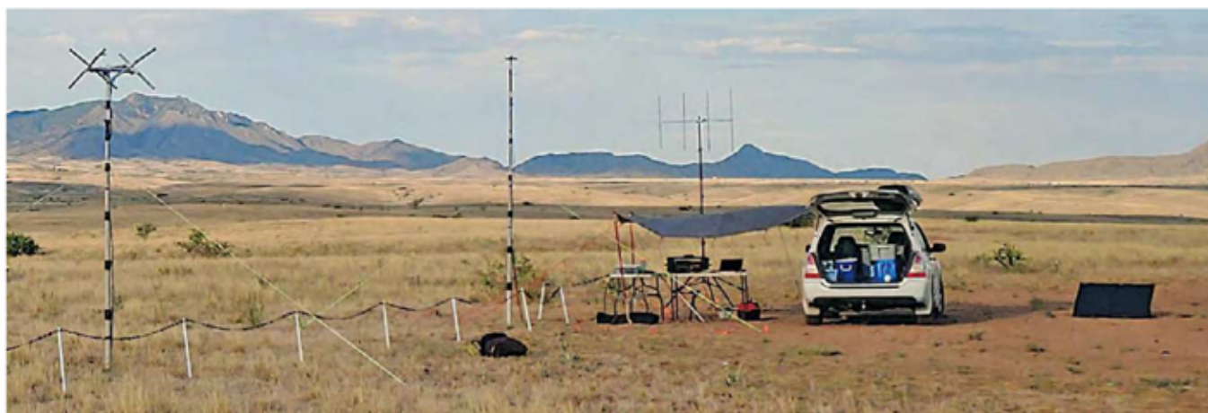
Curt Laumann, K7ZOO, set up his 2020 ARRL Field Day station just outside of Sonoita, Arizona, powered entirely by solar power. In the foreground are his 2-meter and 70-centimeter Lindenblad antennas, which he used for satellite contacts. [Curt Laumann, K7ZOO, photo]
