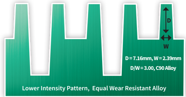
Maximize KM/Rev with Thinner Bars while Maintaining Hydraulic Capacity and Plate Life
