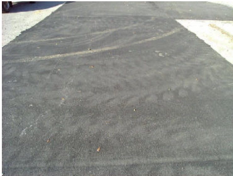
Figure 3. PCMO surface in October 2012. Some scuffing of the surface from the tank testing in August 2008 is apparent.
