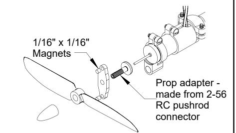
Glue 1/16" x 1/16" magnets in the magnet bar. Make sure the polarity of each magnet is the same. Fit the prop adapter to the motor shaft. Use red Locktite to secure the prop adapter. When the Locktite is set, slide the magnet bar onto the prop shaft. Make sure the orientation is such that the magnet bar is attracted to the magnet in the magnet holder. Slide the prop onto the prop shaft and secure it with the prop nut.
