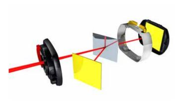
The differentiator behind single-laser technology is located in the sensor housing: A single laser beam is split into two, hitting two separate detectors with an unvariable distance.
