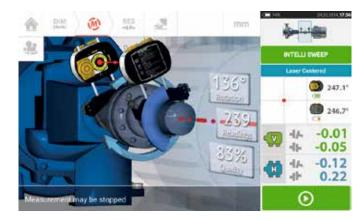
The intuitive user interface supports the user from the beginning to the results stage. In real time, the user can survey the intelliSWEEP® process, the measurement quality, and also the physical positions in horizontal and vertical directions of the machine during the entire alignment process.
