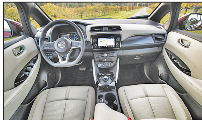
The new LEAF comes with the e-Pedal, which allows the driver to accelerate, decelerate or stop by using the pedal alone.
