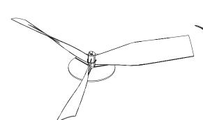
7. When the glue is set use a piece of thread or high strength light fishing line like Spider Wire to lash the hub joint. Pull the line through the holes in each blade near the hub and glue. Make several wraps around the hub.
