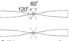
2. Using a razor saw, or other suitable cutting tool, cut each prop hub as shown. The included angle is 120 degrees or as close to that as you can eye ball. The angle can be a little off without causing a problem.
