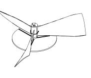
8. When the glue is set on the hub lashing, the free wheel ramp on the front of the prop assembly can be cleaned up with a file or Dremel style tool.
