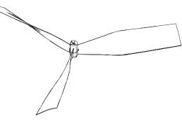
9. This completes the basic assembly of the prop. If the prop will not have a spinner, remove the plywood disk and file the brass tubing to be flush with the prop hub.
