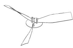
6. Glue each prop blade to the brass tubing using the lines on the disk as alignment marks. Don't worry if the hub joint is not perfect.
