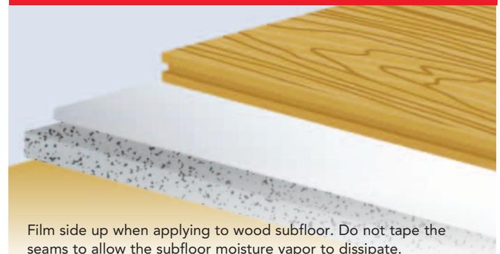
Film side up when applying to wood subfloor. Do not tape the seams to allow the subfloor moisture vapor to dissipate.
