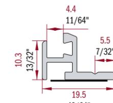
ALUMINUM LOWER PROFILE FOR CREATING LATERAL AND REAR CLOSURES FOR THE SHELVING STRUCTURE.
