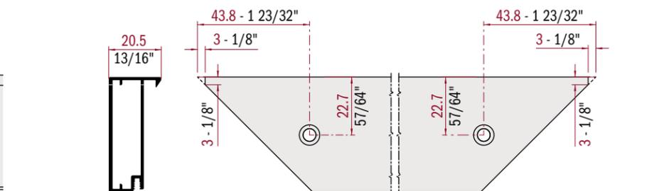
**WARNING:** It is possible to assemble the 2465 sections with the standard 45° cut using squares and screws; when adding the Plastic Corner Bumper CSP0081 an additional 3mm 90° cut is required on the edge of the sections.
