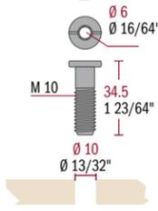
DRILLED SCREW M10 FOR SOCKET
