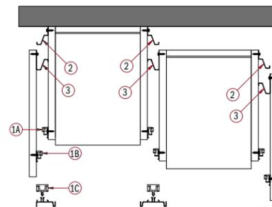
We recommend using screws for wood Ø 3,5 - Ø 9/64"
