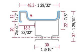
"GOLA" VERTICAL ALUMINIUM SPACER CHANNEL PROFILE FOR CABINET
