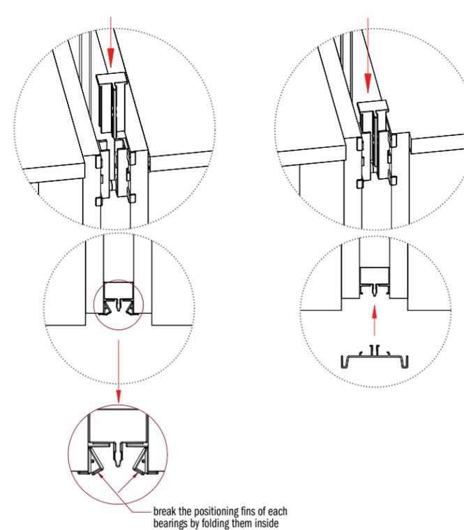
break the positioning fins of each bearings by folding them inside
