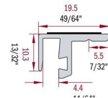
UPPER PROFILE IN ALUMINUM FOR THE CREATION OF LATERAL AND REAR CLOSURES FOR THE SHELVING STRUCTURE.
