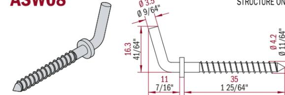
ANGLED SCREW FOR HANGING THE SHELF STRUCTURE ON THE WALL
