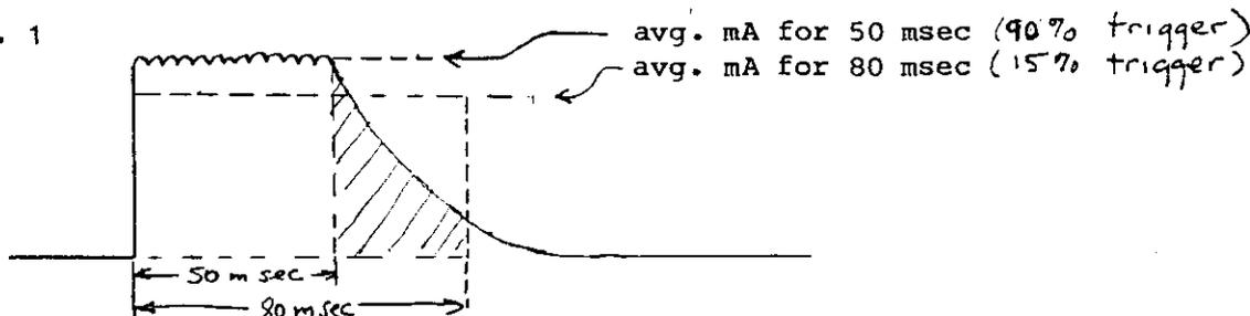
With the generator set for a 50 msec exposure, and the waveform shown in figure 1, if the trigger level is set high (90%) the mA will be integrated for 50 msec. With the trigger level set low, it will be integrated for roughly 80 msec. When the average mA is calculated, since the cross hatched area has a reduced value, the displayed mA for low trigger will be almost 20% less than for the high trigger value.
