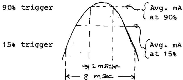
Most people don't realize that the mA will also vary with trigger level, and can read about 50% high at 90% trigger.
