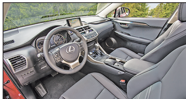
For passenger comfort, the couple distance between the front and rear hip points is 37.9 inches, and the high-roof design provides ample headroom.
