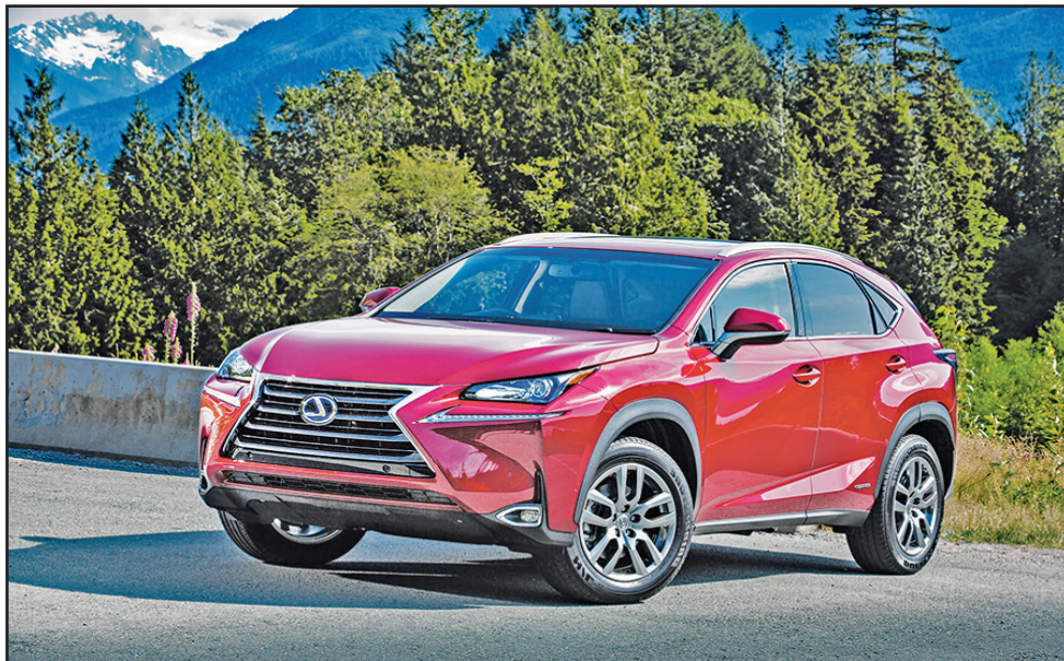
The hybrid features the Lexus E-Four proactive AWD system with an electric motor to drive the rear axle, while the front axle is propelled by gasoline or electric power, or a mixture of both.
