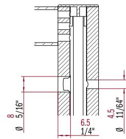
To drill the double diameter hole:
