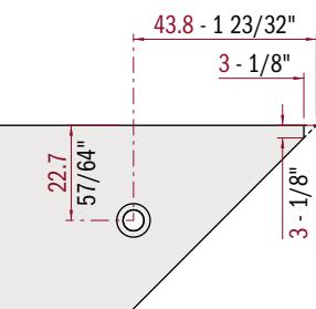
**WARNING:** It is possible to assemble the 2465 sections with the standard 45° cut using squares and screws; when adding the Plastic Corner Bumper CSP0081 an additional 3mm 90° cut is required on the edge of the sections.
