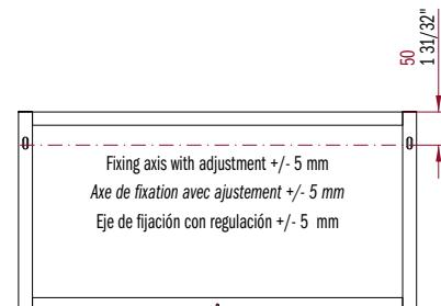
Once adjusted, the structure must be secured to the wall with a normal screw in the hole made in the crossbar.
