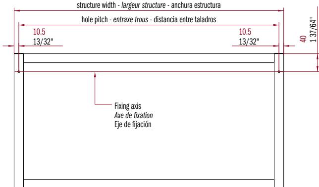
Drill through holes, diameter 4.5 mm, on the 7711 profile in the position shown on the drawing.
