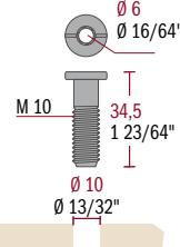
DRILLED SCREW M10 FOR SOCKET
