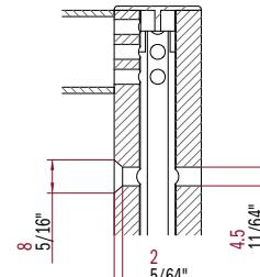
**TYPE B** - Double diameter hole. Invisible screw. Visible hole diameter 8 mm. Total adjustment 1 mm. Secure fixing to the wall.
