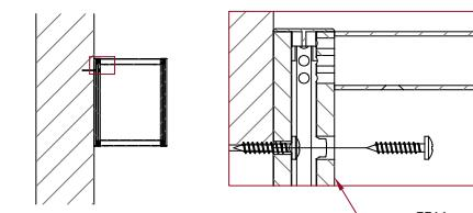
**IMPORTANT:** to cover the head of the screw or the hole diameter 8 mm, apply adhesive cover caps (not included).
