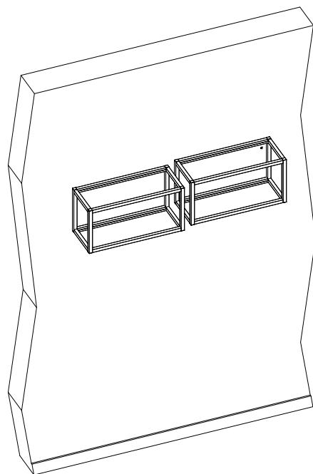
Supporting materials: concrete. Solid or semi-solid bricks. Solid block or light cable concrete. Aerated concrete. Plasterboard. Natural stone. Chipboard panel. Solid gypsum panel.
