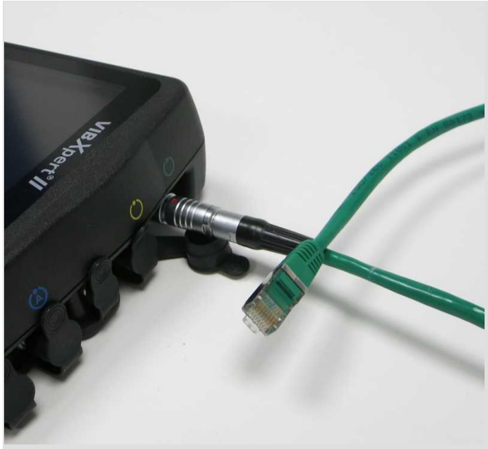
Ethernet cable connected to VIBXPART II
