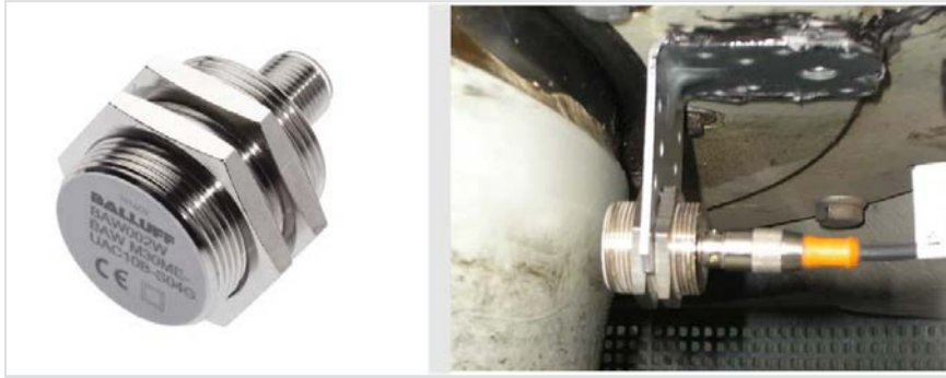
Displacement sensor for use with a stationary measurement system (left); Detection of radial movement in a shaft (right)
