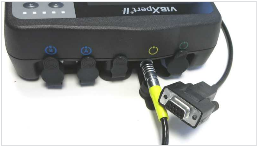
Serial PC cable connected to VIBXPERT II
