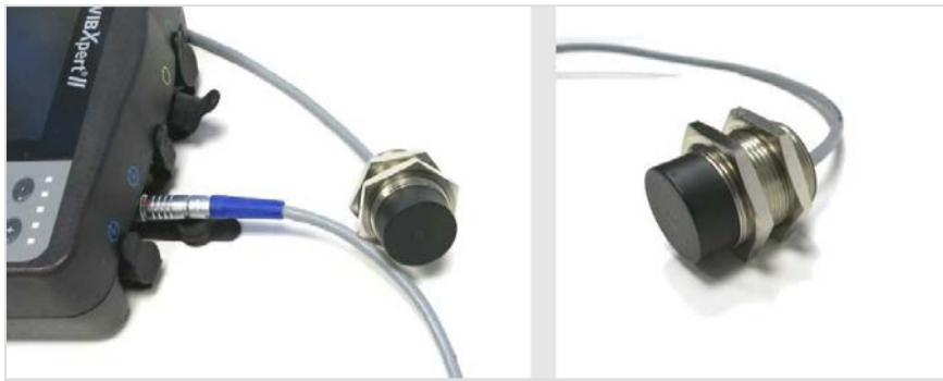
Displacement sensor connected to VIBXPART II
