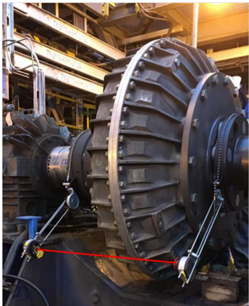
Chain-type bracket for large diameter, ALI 2.460
