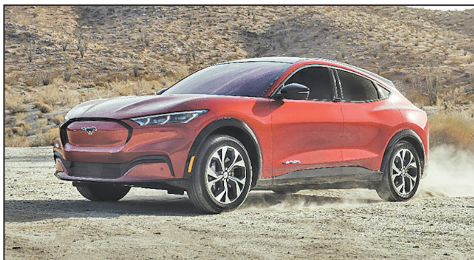
The Mach-E gets 105 City, 93 highway, and 105 Combined MPGe. It weighs between 4,400 and 4,900 pounds, depending on battery size and rear- or all-wheel drive configuration.
