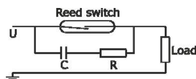
Protection with a RC suppressor for a.c. current and inductive load load.
