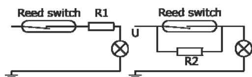
Lamp load with series or parallel resistance to the reed switch.
