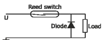
Protection with a diode for d.c. current and inductive load.
