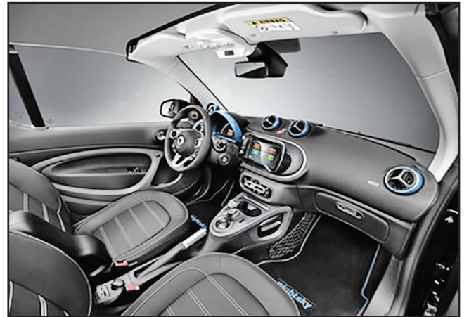
Like a nut, the interior is protected from harm by a rigid shell: the tridion safety cell.
