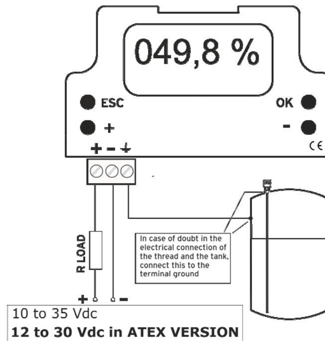
The maximum resistance of the line in serial depends on the power supply. These values have to be bear in mind for the good run of the NMC.
