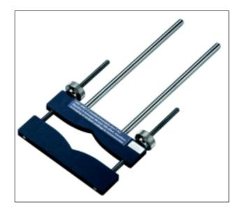
Only 8 mm (5/16") thick, this bracket offers an ideal solution to those occasional tight squeezes between coupling and machine housing. The case includes one complete set for both sides of the shaft or coupling, including various threaded rods and quick-mounting slip nuts. For shafts of diameter up to 6 5/16".
