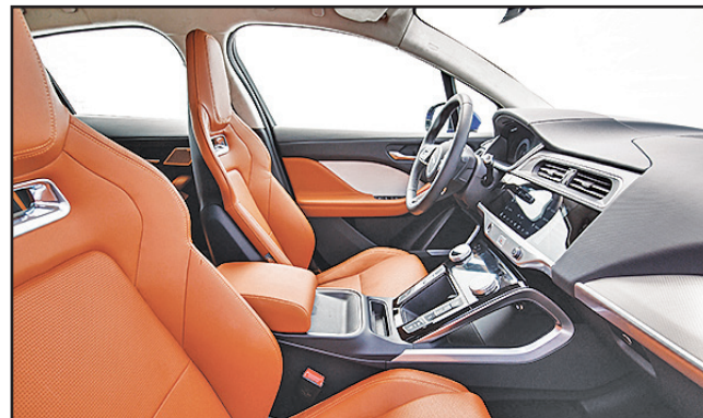
To maintain the calm interior, the i-Pace features acoustic laminated glass on the front windows and windshield, reducing outside noise.
