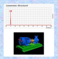
Hold-down bolts need to be torqued each time in the right sequence to avoid that the bolts are too tight or too loose. Otherwise, fasteners can break, or increased vibration occurs. The looseness is usually picked up by the vibration team. (1x and occasionally its harmonics as shown in image to the left image courtesy of Mobius Institute).
