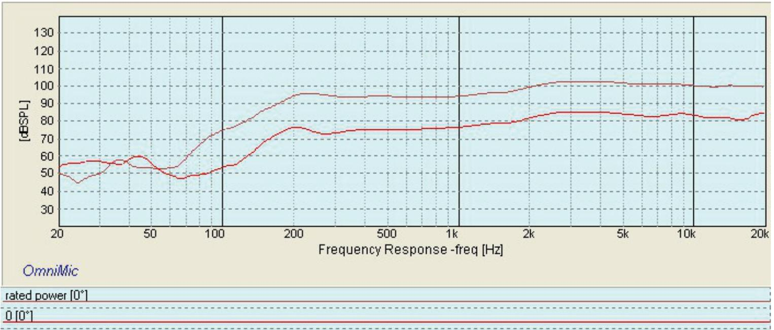
Eros cube speaker 1 watt vs max output full range, free field measurement, smoothing 1/6 octave
