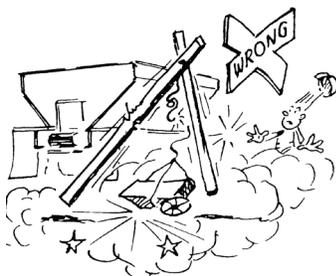
use lifting device that is properly rated to lift the equipment. Do not lift loaded spreader. NEVER LIFT EQUIPMENT OVER PEOPLE.
