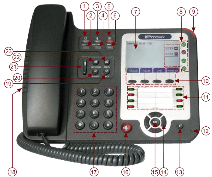
Figure 4 IPitomy IP410 Buttons and Hardware Definitions
