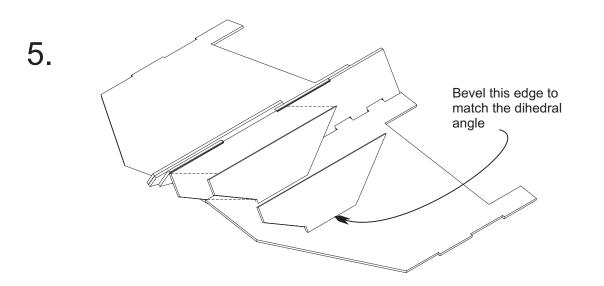
Glue 2 fuselage doublers to each side of the fuselage. Use the sloped front edge as a location guide. The doublers will extend forward of the fuselage sides. Bevel each doubler to fit the wing dihedral angle.
