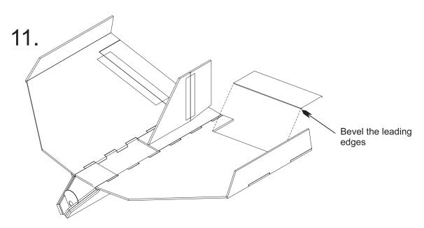
Install the elevators and rudder with hinge tape. Bevel the leading edges before installing.
