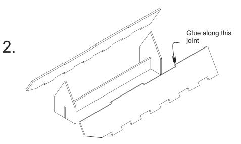
Assemble the two fuselage sides as shown upside down over the assembly jig. **Do not glue the sides to the jig**. Glue the sides together at the bottom joint.
