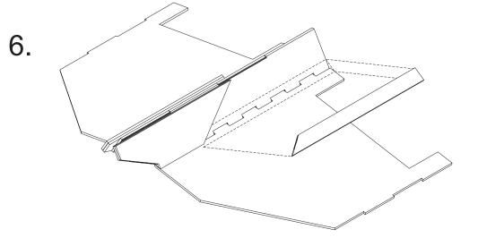
Glue a dihedral brace to each side of the fuselage and corresponding wing panel. The pieces are set at an angle so the edges touch the fuselage side and wing panel with a space between the brace and the fuselage/wing joint. The edges do not need to be beveled.
