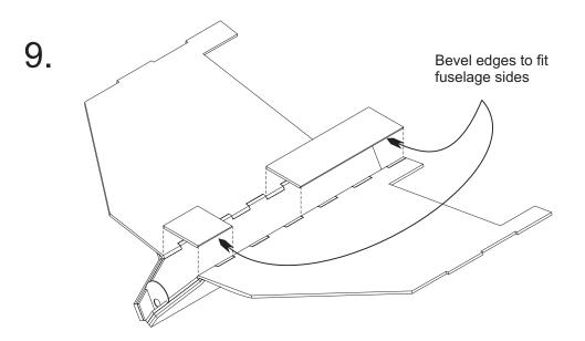
Glue the fuselage top pieces in place as shown. Bevel the edges to fit the fuselage sides.
