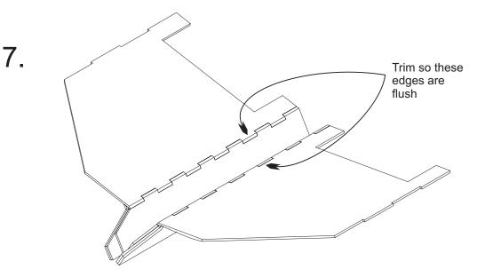
Remove the model from the assembly jig. Trim the wing to fuselage joints so the edges are flush.
