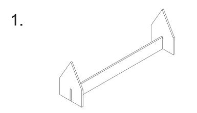
Assemble the fuselage assembly jig components as shown.
