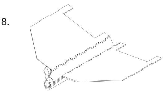
Glue the 1/8" plywood motor mount to the front of the fuselage sides and the inside faces of the doublers. Also glue the forward fuselage side pieces in place in front of the motor mount.
