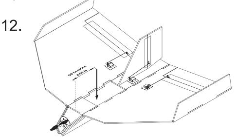
Install the servos, control horns, and pushrods. Use of 1/32" plywood plates under the servos is recommended. Also install the receiver, ESC, and motor to complete the assembly.
