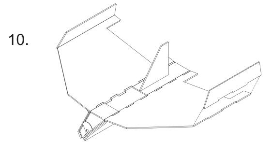
Glue the tip fins and the main fin in place. The tip fins are perpendicular to the wing panels. That makes them look slanted when the model is viewed from the front. The main fin is centered on the rear fuselage top piece and the forward edge is flush with the forward edge of the rear fuselage top piece.
