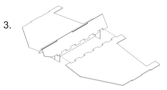
With the fuselage resting on the assembly jig, glue each wing panel in place. The tips of each panel rest on your building surface. The dihedral will be automatically set to the correct amount.
