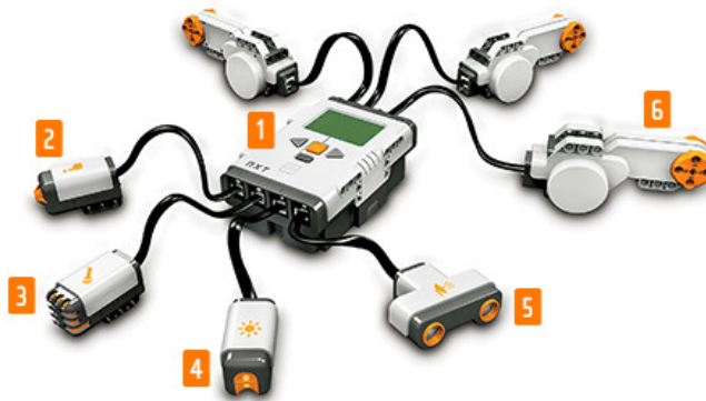
Fig. 1. The Lego Mindstorms NXT. In the center, the NXT brick 1. Above, the three servo motors 6. Below, the four sensors: touch 2, sound 3, light 4 and ultrasonic 5.
