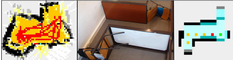
Fig. 8. Example of an environment map representation. In the left side, the map obtained by the first approach, in the middle, the real environment and in the right side the map obtained by the second approach.
