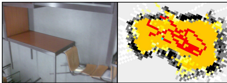
Fig. 6. Example of an environment map representation. In the left side, the real environment and in the right side the map obtained by the first approach.
