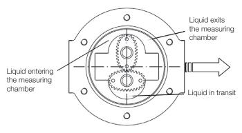
Positive displacement flowmeters are an inexpensive means to accurately meter many high viscosity liquids as high as one thousand centipoise. The appropriate meter must be sized to accommodate the pressure drop across the primary measuring elements (oval rotors) and to not exceed the maximum pressure drop of the meter. The flowmeter should be installed so that the rotor shafts are in the horizontal plane.
