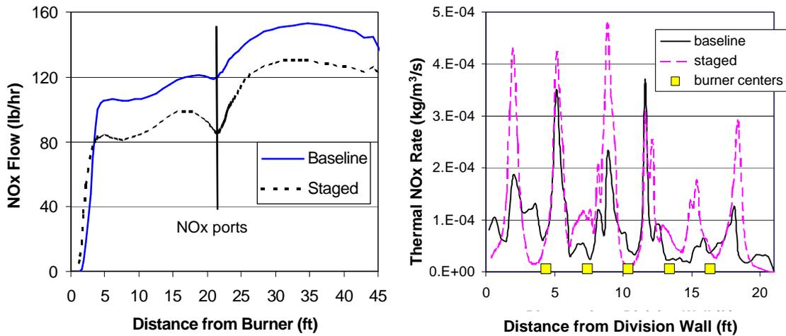
**Figure 9. Plots of predicted downward NOx flow vs. distance below the burners (left) and predicted thermal NOx formation rate vs. distance from the furnace side wall at the NOx port elevation (right).**
