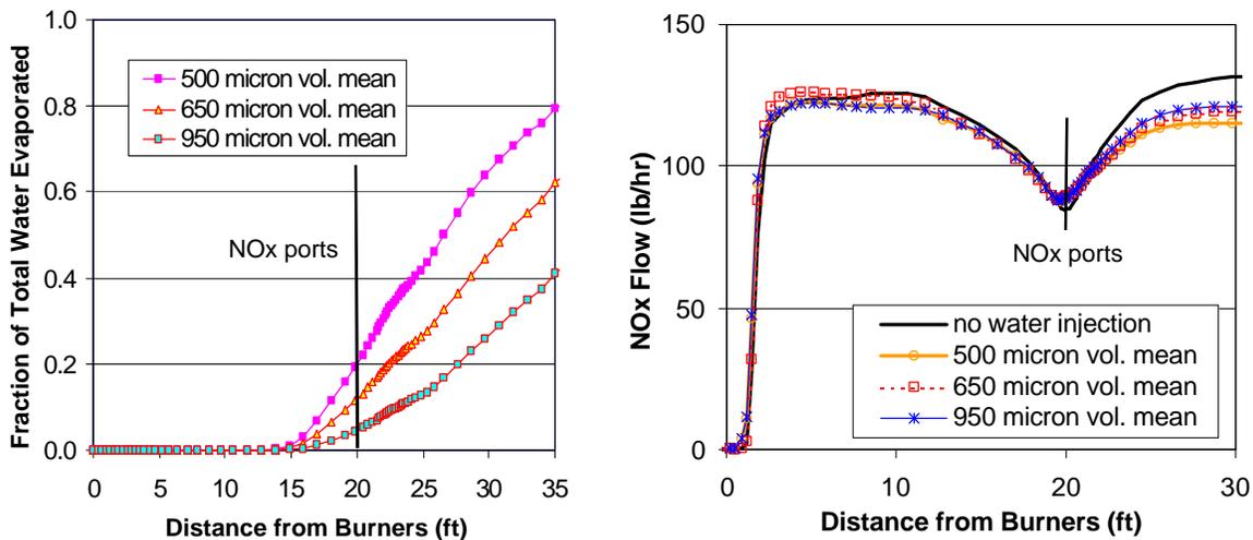
**Figure 11. Plots of the cumulative fraction of injected water evaporated (left) and downward NO<sub>x</sub> flow (right) vs. distance below the burners.**
