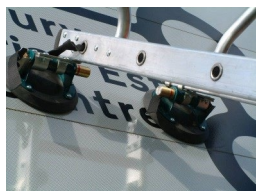
Suction bracket to work on signage, glass ect.
