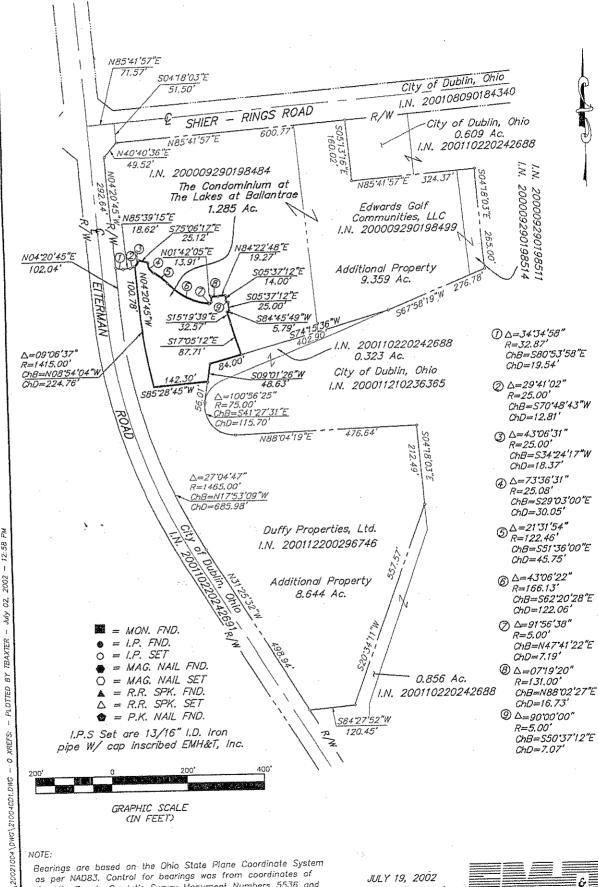
Bearings are based on the Ohio State Plane Coordinate System as per NAD83. Control for bearings was from coordinates of Franklin County Geodetic Survey Monument Numbers 5536 and 7752, having a bearing of South 85'44'20" East, established by the
