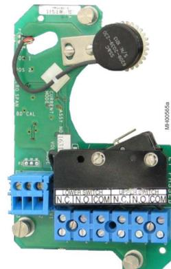
**Mechanical Limit Switch and 4-20 mA Board**
