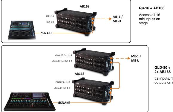
32 inputs, 16 outputs on stage
