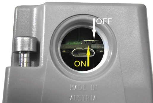
Fig. 11 Bus termination resistor
