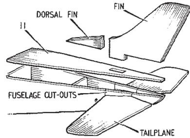
CEMENT TAILPLANE IN POSITION AND REPLACE FUSELAGE CUT-OUTS. ADD PART 11, CEMENT HALVES OF FIN AND DORSAL FIN TOGETHER AND CEMENT IN PLACE **6**
