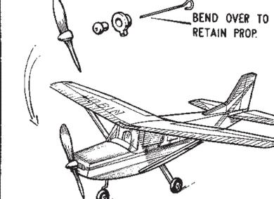
CHECK WINDSCREEN FOR FIT AND CEMENT CAREFULLY IN PLACE, PINNING IN POSITION WHILST DRYING. ASSEMBLE NOSE UNIT AND CHECK FOR FIT IN FUSELAGE. **8**
