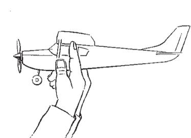
MODEL SHOULD BALANCE AT ABOUT 40% OF WING CHORD AS SHOWN. PLASTICINE MAY BE ADDED TO NOSE OR TAIL TO CORRECT IF NECESSARY. **4**
