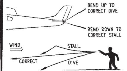
TEST FOR GLIDE ON A CALM DAY. LAUNCH GENTLY AND OBSERVE FLIGHT PATH. CORRECT FAULTS BY BENDING ELEVATORS OR BY ADDING WEIGHT IF REQUIRED. **5**
