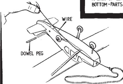
INSTALL RUBBER MOTOR BY MEANS OF A PIECE OF WIRE OR THREAD INSERTED FROM THE TAIL END OF FUSELAGE. SECURE AT REAR END WITH 1/8" DOWEL PEG. **2**
