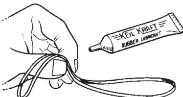
PREPARE RUBBER MOTOR FOR FLYING BY LUBRICATING WITH RUBBER LUBRICANT OR CASTOR OIL. CAREFULLY RUN IN, MOTOR SHOULD TAKE APPROX. 200-250 TURNS. **1**
