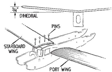
CEMENT WINGS IN POSITION, PINNING IN PLACE UNTIL DRY. CHECK THAT DIHEDRAL IS CORRECT - 3/4" UNDER EACH WING TIP AND THAT WING FITS SNUGLY IN PLACE **2**
