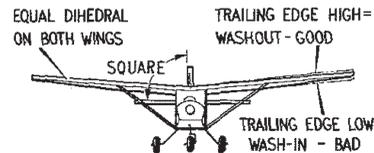
CHECK THAT ALL SURFACES LINE UP TRUE WHEN VIEWED FROM THE FRONT OR FROM ABOVE. WINGS SHOULD BE STEAMED TO INCORPORATE SLIGHT WASHOUT AT TIPS. **3**
