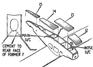
CEMENT UNDERCARRIAGE IN PLACE TO FORMERS 4 AND 7, AND REINFORCE WITH A SKIN OF CEMENT. ADD FUSELAGE BOTTOM-PARTS 12, 13, 14 AND 15 **5**
