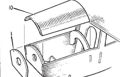
ADD FUSELAGE PART NO. 10 CHAMFERING EDGES OF 10 TO ENSURE A PERFECT FIT WITH FUSELAGE SIDES. NOW FIT FRONT FORMER, PART 1. **4**
