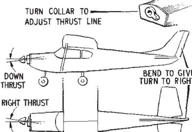
COMMENCE FLYING UNDER POWER WITH 50 TURNS ON MOTOR. ADJUST THRUST LINE TO PREVENT STALLING. CEMENT COLLAR IN PLACE WHEN BEST SETTING IS FOUND. **6**
