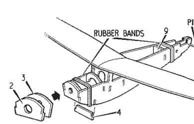
CEMENT FORMERS 2 AND 3 TOGETHER. JOIN FUSELAGE AT NOSE AND TAIL, FITTING FORMERS 2, 3, 4 & 9. HOLD TOGETHER WITH PINS OR RUBBER BANDS UNTIL SET. **3**
