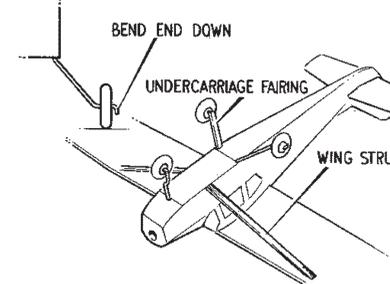
FIT WHEELS TO UNDERCARRIAGE LEGS AND RETAIN BY BENDING DOWN END OF AXLES. CEMENT UNDERCARRIAGE FAIRINGS TO LEGS AND ADD WING STRUTS. **7**
