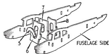
CEMENT FUSELAGE SIDES TO FORMERS 5, 6, 7 AND 8. MAKE SURE THAT ASSEMBLY IS SQUARE AND THAT SIDES AND FORMERS LINE UP CORRECTLY, THEN LEAVE TO SET **1**
