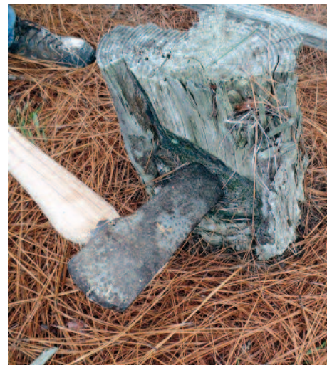
An 1800's box ax chopped out a cup in 100 year old pine stump with box face to catch the pine tar.
