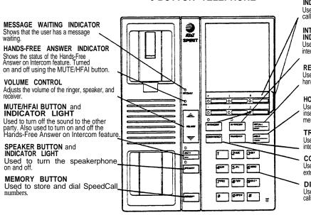
LINE BUTTONS (1-6) and INDICATOR LIGHTS Used for placing and receiving outside calls.
