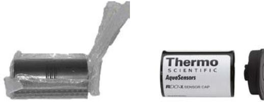
4. Align the arrow on the cap with the index mark on the sensor and firmly press the cap onto the sensor, without twisting, until it seals over the probe body.
