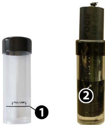
2. Completely submerge the foil of the sensor, making sure that the temperature thermistor is also completely submerged under the surface of the solution. Do not allow the foil to rest completely on the bottom of the calibration chamber. Leave at least ½-inch between the surface of the foil and the bottom of the chamber.
