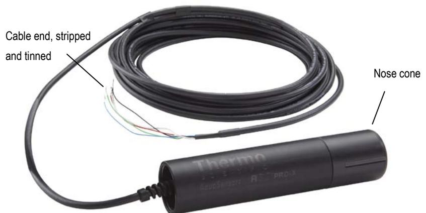
The System is used for continuous monitoring of dissolved oxygen from 0 ppm to 20 ppm. The system also measures temperature from 0°C to 100°C. The optical sensor head is pre-calibrated and the zero is factory set. The sensor retains calibration values and does not require a new calibration when the system is connected to a new AV38 Display Unit, AquaPro, PC, or PLC.
