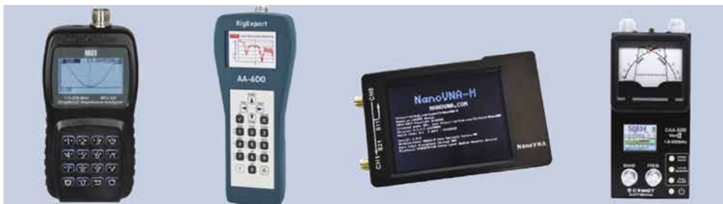
Above, left to right: An MFJ analyzer doing a frequency sweep to find the lowest SWR. ■ A RigExpert AA-600 analyzer doing an SWR sweep through a broad range of frequencies. ■ The NanoVNA sells for less than $100. ■ The Comet CAA-500 Mark II analyzer offers a mechanical meter and a graphic display.
