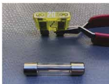
Figure 5: Replacement fuses — glass tube style (bottom) and automotive blade style (top). You can see that the wire inside each of these fuses is intact.
