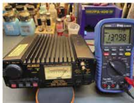
Figure 3: Power supply outputs correct voltage.
