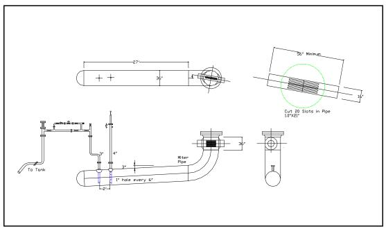
The width of each slot is 2.5 times pipe wall-thickness, terminated on both ends by a half circle to reduce stresses. Total slot-area must be at least twice the outletnozzle area. There are an odd number of slots in each quadrant of the pipe (with the center of each set located at  $0^{\circ}$ ,  $90^{\circ}$ ,  $180^{\circ}$ , and  $270^{\circ}$ ). The slots are located 2.5 pipe widths apart. With this configuration the slot length is:
