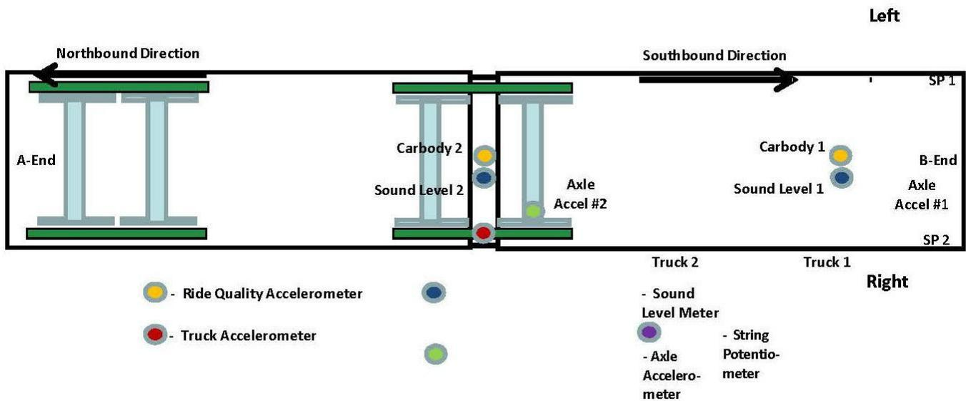
Figure 2. Sensor Layout Used For Test Vehicles
