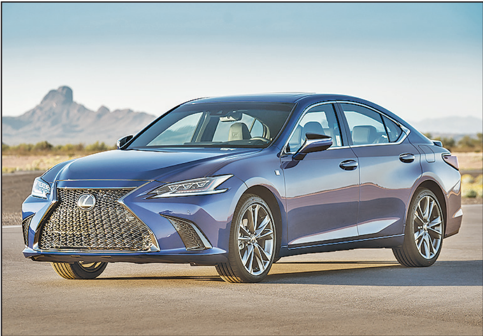
To generate higher EPA miles-per-gallon numbers, Lexus puts a 2.5-liter four-cylinder in with a high-density motor and nickel-metal-hydrate battery which together put out 215 horsepower.
